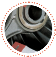
Needle bearing in both connecting rod eyes
